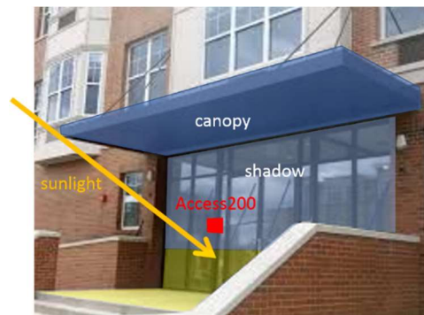
Figure 4: Top view of building entrance (left) with angle-mounted Access200 oriented to avoid direct sun. Access200 conveniently faces entering subjects in this orientation. Photo of same building entrance (right).
